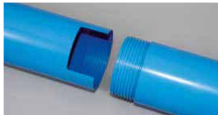
FJTT Flush joint trapezoidal thread according to work standards. Threads are cut into the wall of pipe : • Pitch 6 mm : Ø 113 to 225 • Pitch 12 mm : Ø 250 to 400
