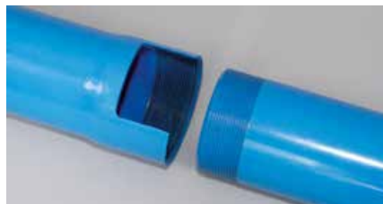
TTSF Trapezoidal thread, blown female socket (according to DIN 4925). • Pitch 6 mm : Ø 113 to 225 • Pitch 12 mm : Ø 250 to 400
