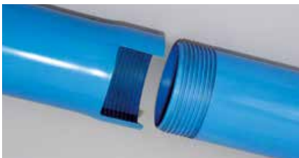
WT Witworth pipe thread according to DIN 2999: cylindrical internal thread and conical external pitch (11 threads per inch).
